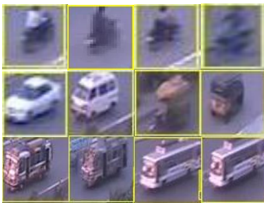
Figure 4: Sample images used to train Neural Networks into three categories. (M, SV, LV)
